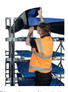
Place the roof insulation into position (inner edge Velcro tabs to the front). Ensure the edges are pulled over the racking.
