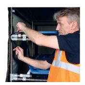
Secure the side panels to the frame at the front using the Velcro straps.
